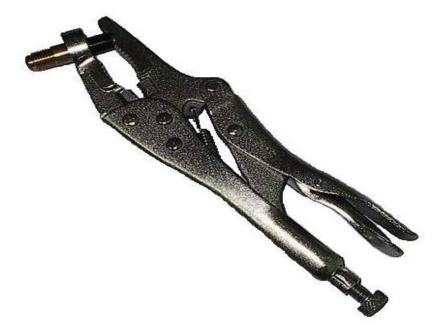
Model 49101 Quick Tap Refrigerant Tool is the fastest and easiest way to evacuate refrigerant before disposal of a unit. Taps onto a refrigerant line for full discharge into recovery unit. Fits from 3/16" to 7/8" OD hard tubing. Needle is replaceable.
